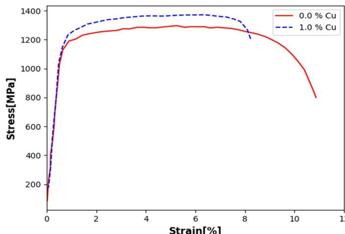
This next graph is data which has been pulled from a paper written by Alexander Gramlich<sup>[4]</sup>. It shows the harmful effects that copper has on the integrity of steel. As seen in the figure, even a small amount of copper can greatly affect the amount of stress that the steel can handle. This can also occur with other metals and alloys, which is why it is important when recycling metals to regulate the number of contaminants.
